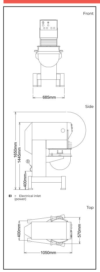
Electric 380-440 V/3N ph/50/60 Hz Supply voltage: **Electrical power max:** 4 kW **Total Watts:** 4 kW Capacity: ISO 9001; ISO 14001 kg/ Performance (up to): Cycle 60 litres Capacity: Key Information: External dimensions, 685 mm External dimensions, 1050 mm Depth: External dimensions, **Height:** 1445 mm **Shipping weight:** 306 kg ISO 9001; ISO 14001 kg **Cold water paste:** with Spiral hook
